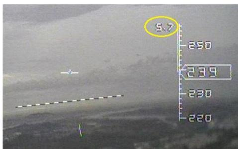
13. AHL (Artificial Horizon Line). AP estimates the current attitude of the plane and simulates a horizon line on the screen.
