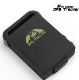
This kind of GPS trackers usually use GSM/WCDMA networks to send its position data continuously. Once the airplane flies high the GPS tracker will try to use maximum output to communicate with the base station. This kind of strong EMI maybe cause the AP malfunctioning. So please keep it as far as possible to AP (at least 20cm).
